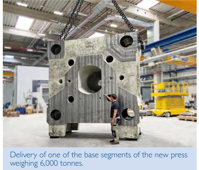
Delivery of one of the base segments of the new press weighing 6,000 tonnes.
